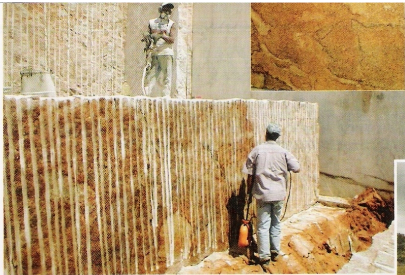
Workers use drills to expose a new bench at the Copper Canyon quarry.
